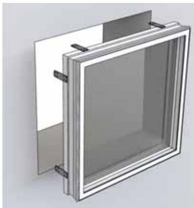
Block frame window installation: Block-frame windows don't have a fin. Installers use plates or screws to fasten the window to its opening.
