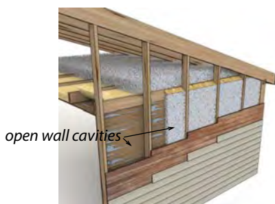
Balloon framed gable: Studs extend above the ceiling allowing convection from the attic.
